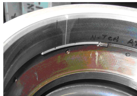
Fig. 14 Test bearing with EDM notch on the outer race
